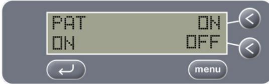
When the ON button is pressed, both the heater and the ultrasonic generator will turn on, irrespective of any other programmed settings.
