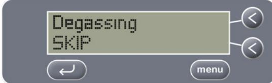
The degassing process is to remove all bubbles from the water as these impede the cleaning performance. Once all of the bubbles have come to the surface, complete the degassing cycle by pressing the ↵ key.
