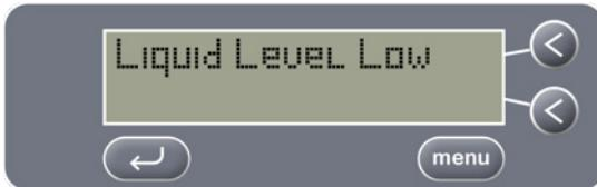
The Grant digital ultrasonic bath will not operate again until the tank is filled to the correct level.
