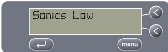
If the liquid temperature exceeds the allowed maximum of 70°C (160°F), the following screen will be displayed
