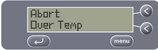
If the internal heater exceeds its allowed maximum, the following screen will be displayed.
