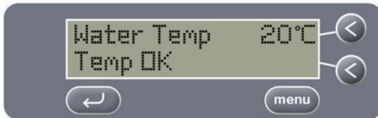
To immediately start the cycle using the already set cleaning parameters, press the ← key.
