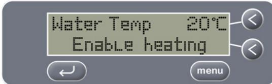
To continue using the Grant digital ultrasonic bath, refill with liquid up to the liquid level sensor and switch the unit off and on again.
