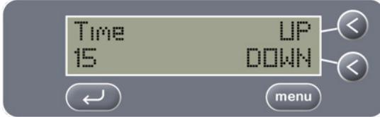
When the desired cycle time has been selected, use the MENU key to move to the next screen. This time setting will be saved until changed again in the Operator menu.
