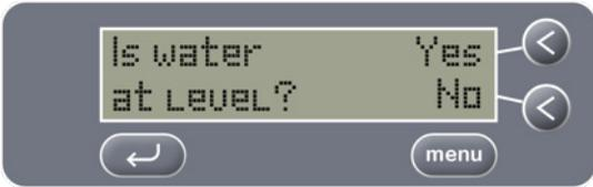
When the level sensor is disabled the liquid set temperature is automatically reduced to 5°C. The set temperature may be increased by entering the MENU system (see page 9).
