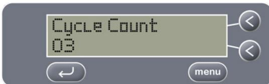
The cycle count shows all cycles which the bath has begun and includes those cycles which are not completed; i.e. those cycles aborted by the operator or because the liquid level was low.
