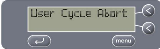
If the Level sensor is set to ON, and the liquid drops below the required level during operation, the cleaning cycle will stop and the following screen will be displayed.
