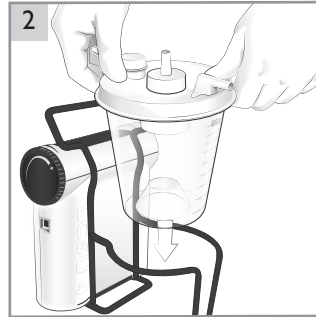
2 Place the Canister into Wire Stand.
